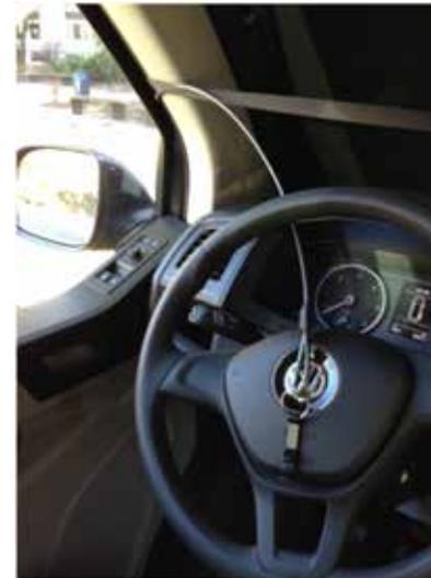
Put the wire rope through the door seal into the inner of the vehicle. The door seal is flexible enough to allow this. Due to the second loop at the end of the wire (and the bottle opener ☺) it is not possible to pull out the wire when the vehicles door is closed.
