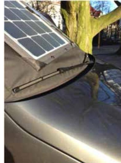
Push the mat down to the bottom of the wind shield. Bring out the wiper and put the wiper onto the mat. The integrated magnets in the isolation mat fix the mat all around the wind shield on the metal of the vehicle. Inside of the vehicle secure the mat with the long strap.
