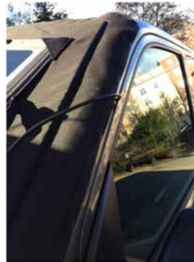
Through the door seal bring the cable inside of the vehicle. The door seal is flexible enough to allow that. Last step is connect the charge controller with the battery by using the 12-Volt plug on the controller or by an individual installation.
