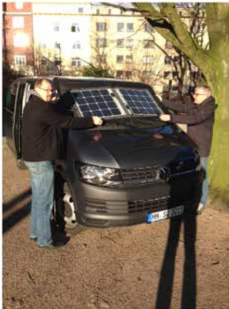
Put isolating mat and module to the wind shield of the vehicle. It is easier to do that with two people.
